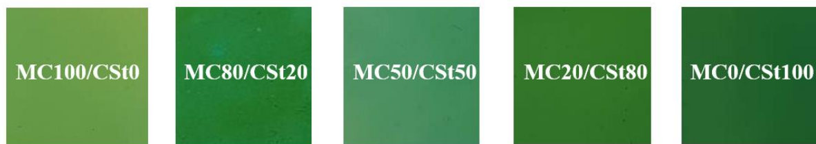
Figure 1 Color appearance of the indicator films prepared from different MC and CSt ratios (MC/CSt: 100:0, 80:20, 50:50, 20:80, and 0:100)
